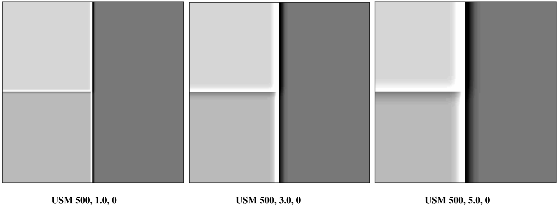
Figure 4. 300% enlargements of the test patches at various USM settings.
